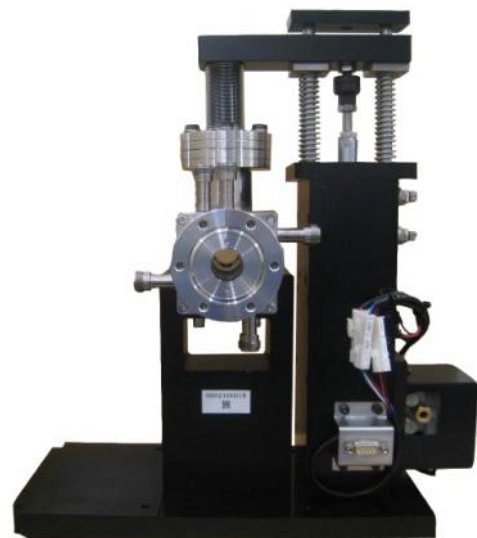
RF Cavity Beam Position Monitor
